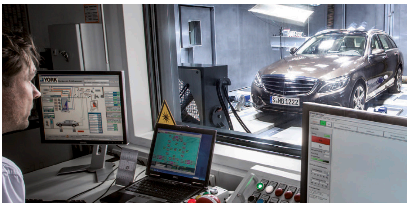
Figure 3-1: Test chamber to measure car cabin emissions
