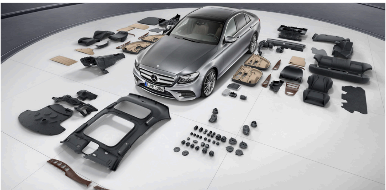
Figure 3-3: Components in the E-Class Saloon produced using renewable materials
