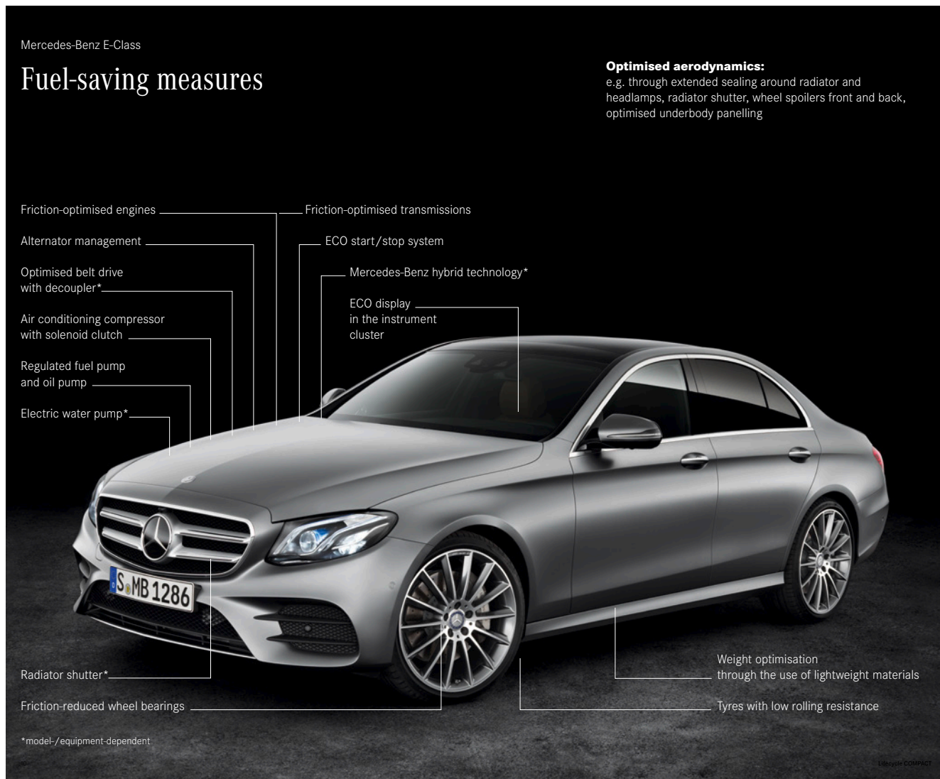
Figure 1-1: Fuel-saving measures for the new E-Class
