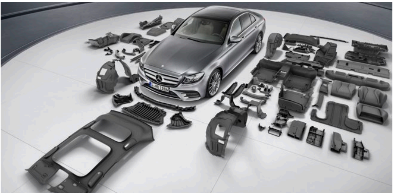
Figure 3-2: Use of secondary raw materials in the E-Class
