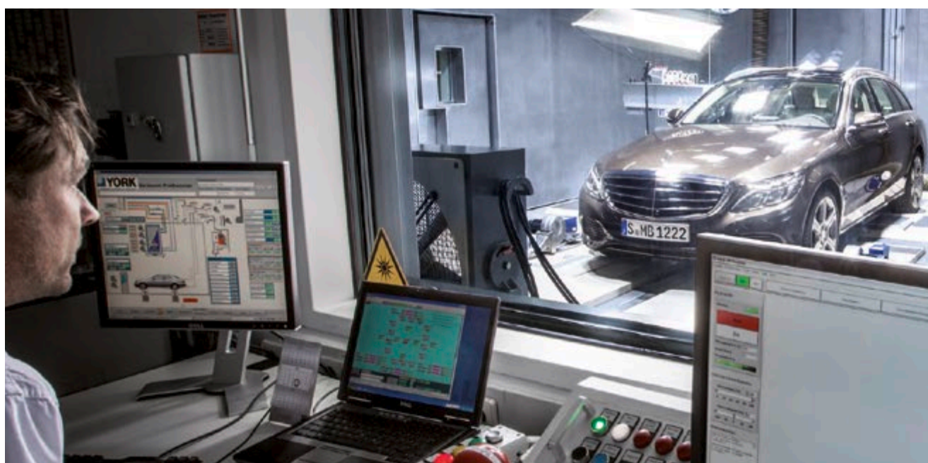
Figure 3-1: Test chamber to measure car cabin emissions
